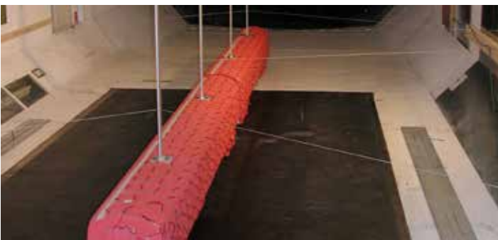
Study of flow / track interaction on a train using PIV (Particle Image Velosymetry) AEA Technologies Rail/ RSSB
