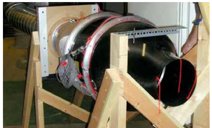
Development of a air jet for Mercedes Ilmor for an F1 car dynamometer
